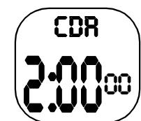
When you finish setting the timer, press SET/LIGHT/STP/RST. To start the timer, press ADV./ST./SPL. To stop the timer and reload the preset time, press SET/LIGHT/STP/RST.
